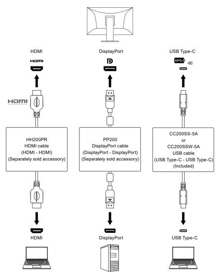
When two PCs are connected to one monitor, you can link the input signals with the USB ports to use a USB device connected to the monitor from both PCs by switching between them. For details, refer to "KVM" (page 27).
