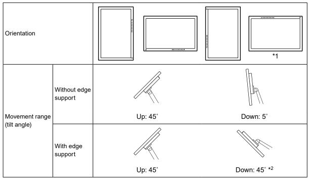
\*1 If you position the monitor facing in this direction, clean the power connector and the surrounding area regularly. If dust, water, oil, or other materials adhere to the device, it can cause a fire.
